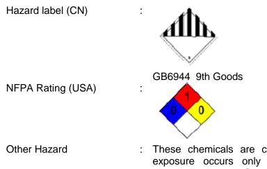
: These chemicals are contained in a sealed can. Risk of exposure occurs only if the battery is mechanically or electrically abused. Contact of electrolyte and extruded lithium with skin and eyes should be avoided.
